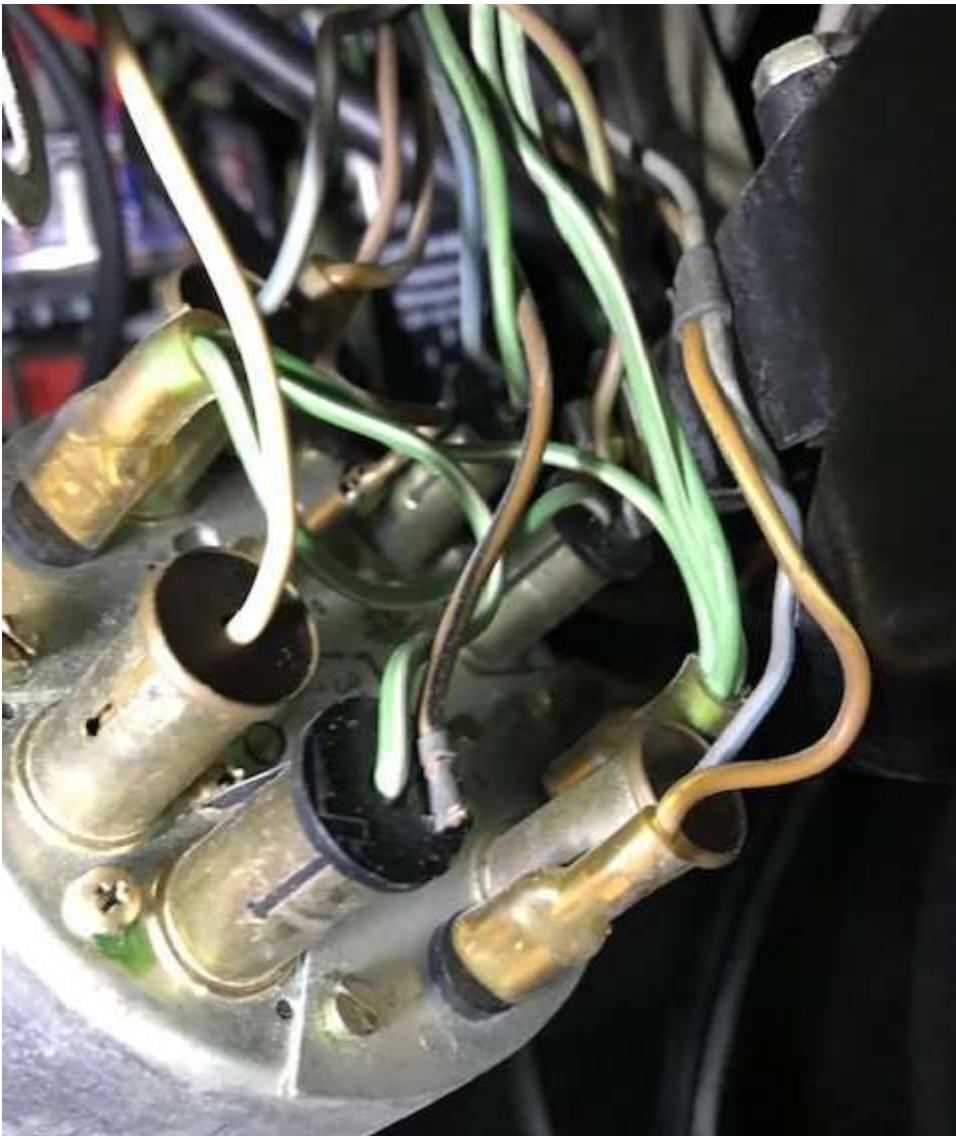
Connections for the Fuel/Temp gauge:
